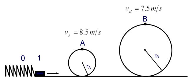
The block has a greater GPE at point B - so since Energy is conserved, it has a smaller KE - hence, a smaller velocity. Note how we don't care how it got there - an elliptical loop would give the same velocity. 38 A spring gun, aimed in the horizontal direction with k = 250 N/m is compressed 0.050 m and released. How fast will a 0.025 kg dart go when it exits the gun?
