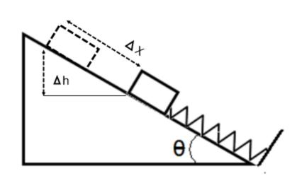
32 A box is held on top of a spring on an inclined plane of angle  $\theta = 31^{\circ}$ . The box is released, compressing the spring. If the spring moves 7.0 m down the plane, how much does its height,  $\Delta h$ , change?
