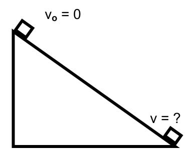
The system will be the block. Since there is no friction, there are no external forces and we can use the Conservation of Energy (the gravitational force is taken care of by GPE). What types of energy are involved here?
