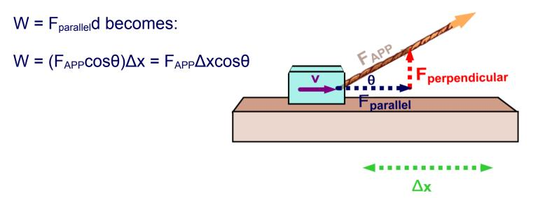
In words, the work done on an object by a force is the product of the magnitude of the force and the magnitude of the displacement times the cosine of the angle between them.
