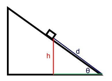
The box starts with no velocity, and after it is pushed up a displacement d, the block slides up, and it momentarily stops before sliding back down.
