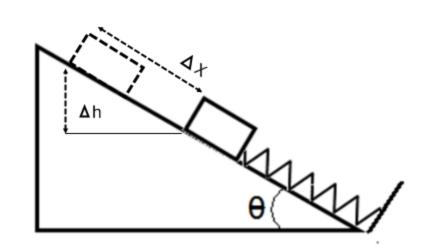
33 A box of mass m is on an inclined plane that makes an angle of  $\theta$  with the horizontal and is in contact with a spring of spring constant k. The box is released, and it compresses the spring an amount  $\Delta x$  before rebounding. In terms of m, g, k and  $\theta$ , what is the value of  $\Delta x$ ?
