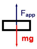
A book of mass, m, is lifted vertically upwards a displacement, h, by an external force (a person) at a constant velocity. How much work does the external force do on the book?
