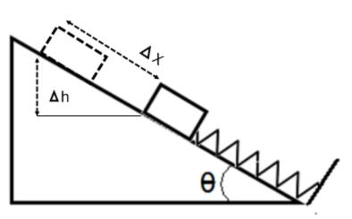
Consider the inclined plane problem that was just worked, but add a spring at the bottom of the incline.
