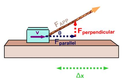
Using trigonometry, we find that  $F_{parallel} = F_{APP} cos \theta$
