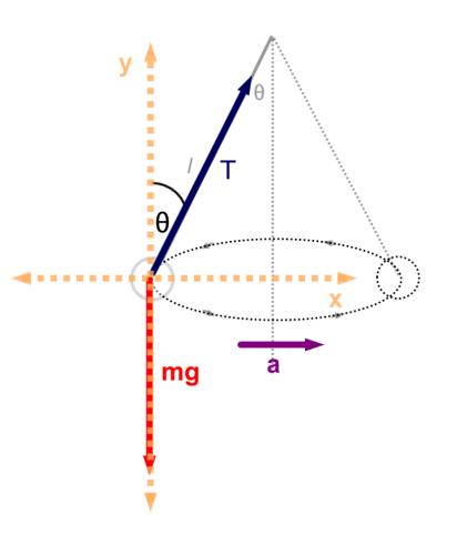
An alternative approach is to solve this as a vector equation using  $\Sigma F$ =ma. (This will work whenever only two forces are present.)
