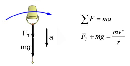
The minimum velocity for a bucket to make it around the circle is achieved when the tension in the string becomes zero at the top of the circle.
