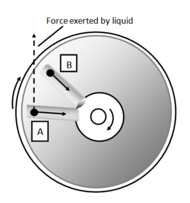
A centrifuge works by spinning very fast. This means there must be a very large centripetal force. The object at A would go in a straight line but for this force; as it is, it winds up at B.
