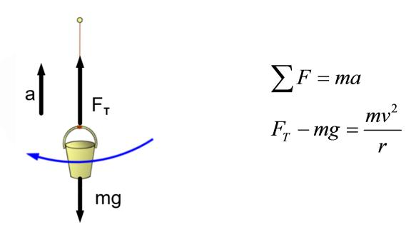
A bucket on a string moving in a vertical circle is also in circular motion. When it is at the top of the circle, there is no force upward. The tension and weight are both down.
