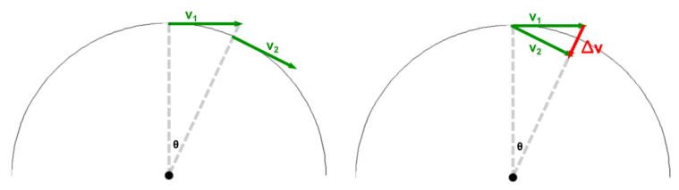
The change in velocity,  $\Delta v$ , shows the direction of the acceleration. In the picture, you can see  $\Delta v$  points towards the center of the circle.
