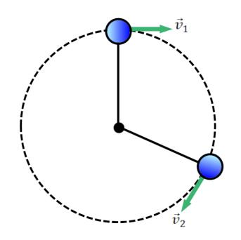
This acceleration is called the centripetal, or radial, acceleration, and it points towards the center of the circle.
