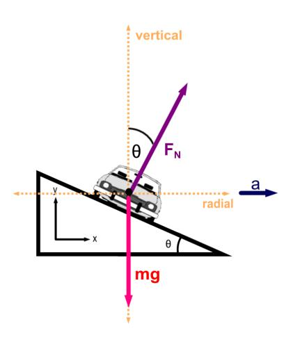
Next, decompose the forces that don't align with an axis,  $F_N$ .
