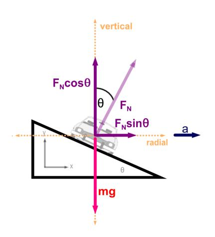
Now let's solve for the velocity such that no friction is necessary to keep a car on the road while going around a curve of radius r and banking angle  $\theta$ .
