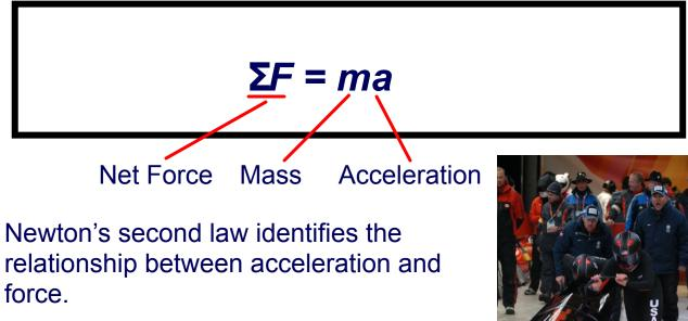
When a net force is applied to an object, the object accelerates.
