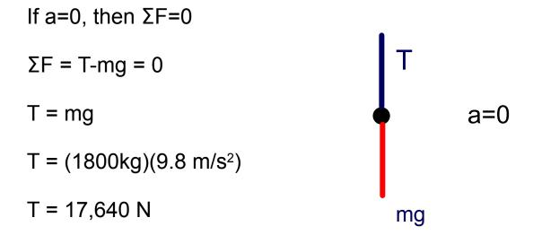
An 1800 kg elevator moves up and down on a cable. Calculate the tension force in the cable for the following cases:
