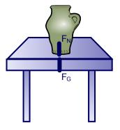
The normal force is exactly as large as needed to balance the force from the object. (if the required force gets too big, something breaks!)
