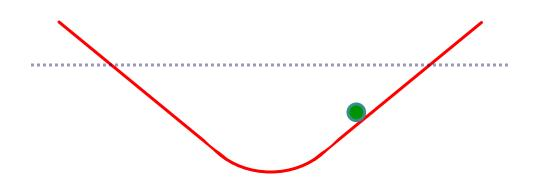
If a ball rolls down one ramp, it keeps rolling up the other side until it reaches the same height.
