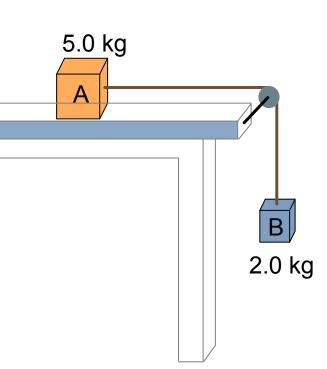
Two boxes are connected by a cord running over a pulley. The coefficient of kinetic friction between box A and the table is 0.2
