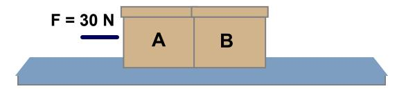
Two boxes are place on a table. A person pushes horizontally on box A with force F = 30.0 N. The boxes A and B have masses of 5 kg and 8 kg. Ignore friction between the boxes and the tabletop.
