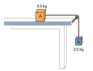
Two boxes are connected by a cord running over a pulley. The coefficient of kinetic friction between box A and the table is 0.2
