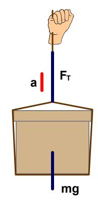
46 A 25 kg lamp is hanging from a rope. What is the tension force being supplied by the rope?
